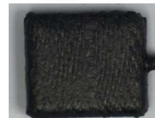
Early development of SiC composite wrap fuel plate sample at GA
