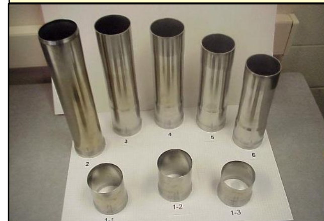
Extruded and flow formed ODS tubing (6")
