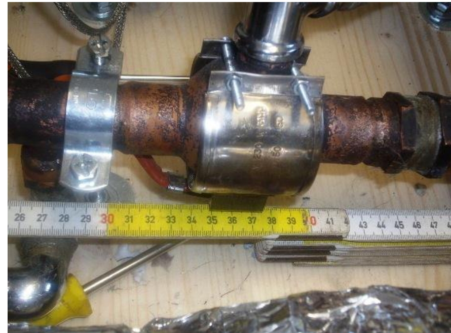
Close-up of the section of the E-Cat which is heated by a clamp-on resistive heater.
